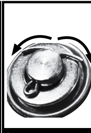
⑨ Slide one washer on each side then insert the split pin through the hole in the end of the axle. Once fully inserted, bend the ends out.
